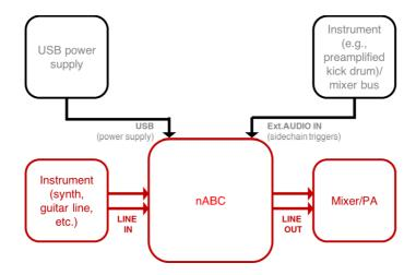
The nABC sidechain can even be triggered with the input line audio signal itself, as a traditional compressor would do. The INT/MIDI/USB Operation Mode should be selected using S/C SELECT.
